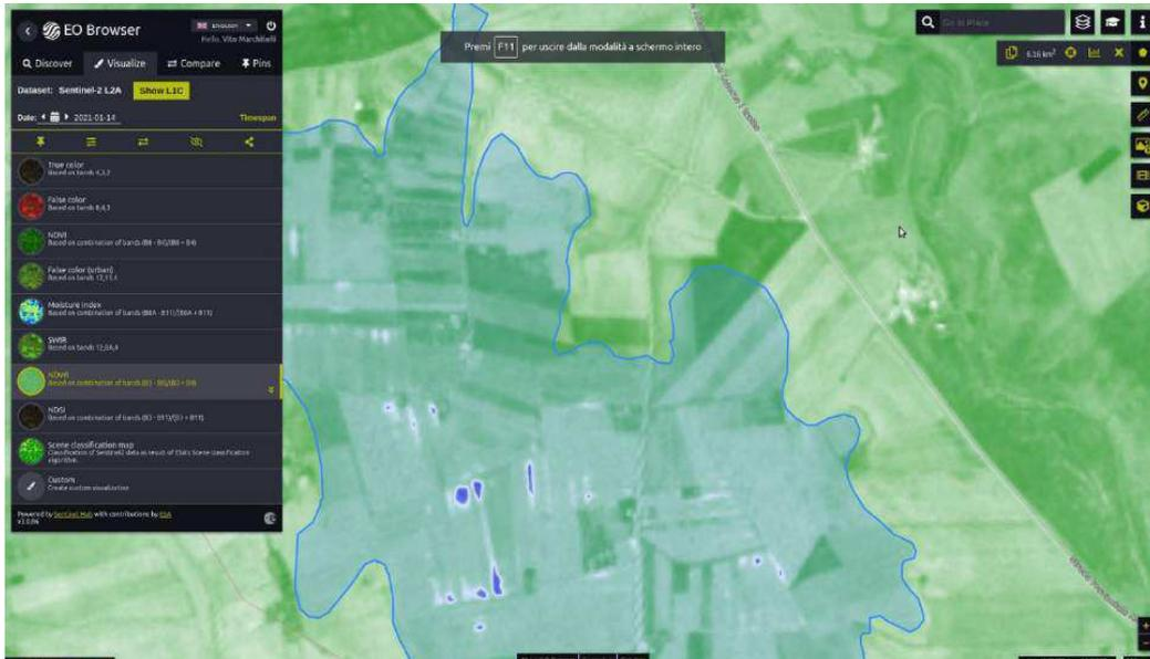
Figura60: Particolare NDWI Based on combination of bands (B3 - B8)/(B3 + B8)
