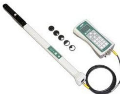
Fig.6 LAI Plant Canopy Analyzer-2200
